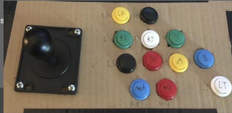
I positioned the buttons and joystick in such a way so that Kyle can efficiently use it based on physical ability.
