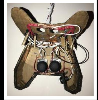
The controller consists of 13 buttons total. Each button had to be soldered because of the restricted amount of space. All of the power wires ran to the bottom of the controller, and the ground wires were organized at the top.
