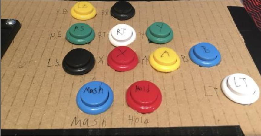
The controller emulates an Xbox controller, the buttons are arranged this way for best use in Destiny 2
