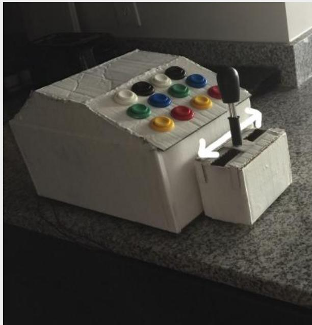
Steer control is made with a potentiometer
